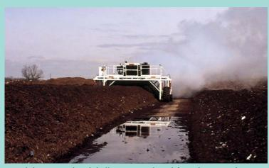
Biosolids are mixed with bulking materials and formed into windrows (long piles).
